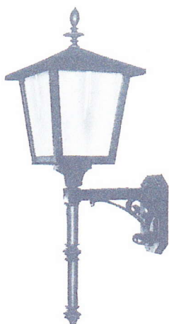
NO. C-404: Height overall 33". Lantern size 11"x19 1/2" Backplate 4 1/2"x9". Wall to center 10 1/4". Maximum Watt. 300W.
